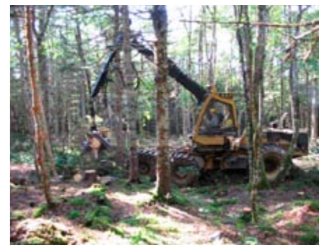
A "single-grip" harvester equipped with eco-tracks that limit damage to the forest floor selectively removes trees in a forest south-east of Monastery, Nova Scotia, managed by NewPage Port Hawkesbury Corporation. Thinning the forest permits more light to penetrate the stand, encouraging faster regeneration of "climax" species such as white pine, red spruce, and yellow birch.
